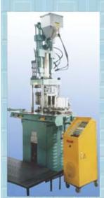
This production line uses plastic injection molding equipment for the injection molding of laminated tube shoulders. This machine uses screw preplastication mold closure completely by hydraulic pressure, double mould alternative forming method, with hydraulic pressure pieces. It is highly efficient in production, easy and safe to work with. It produces smooth and cosmetically high quality shoulders.
